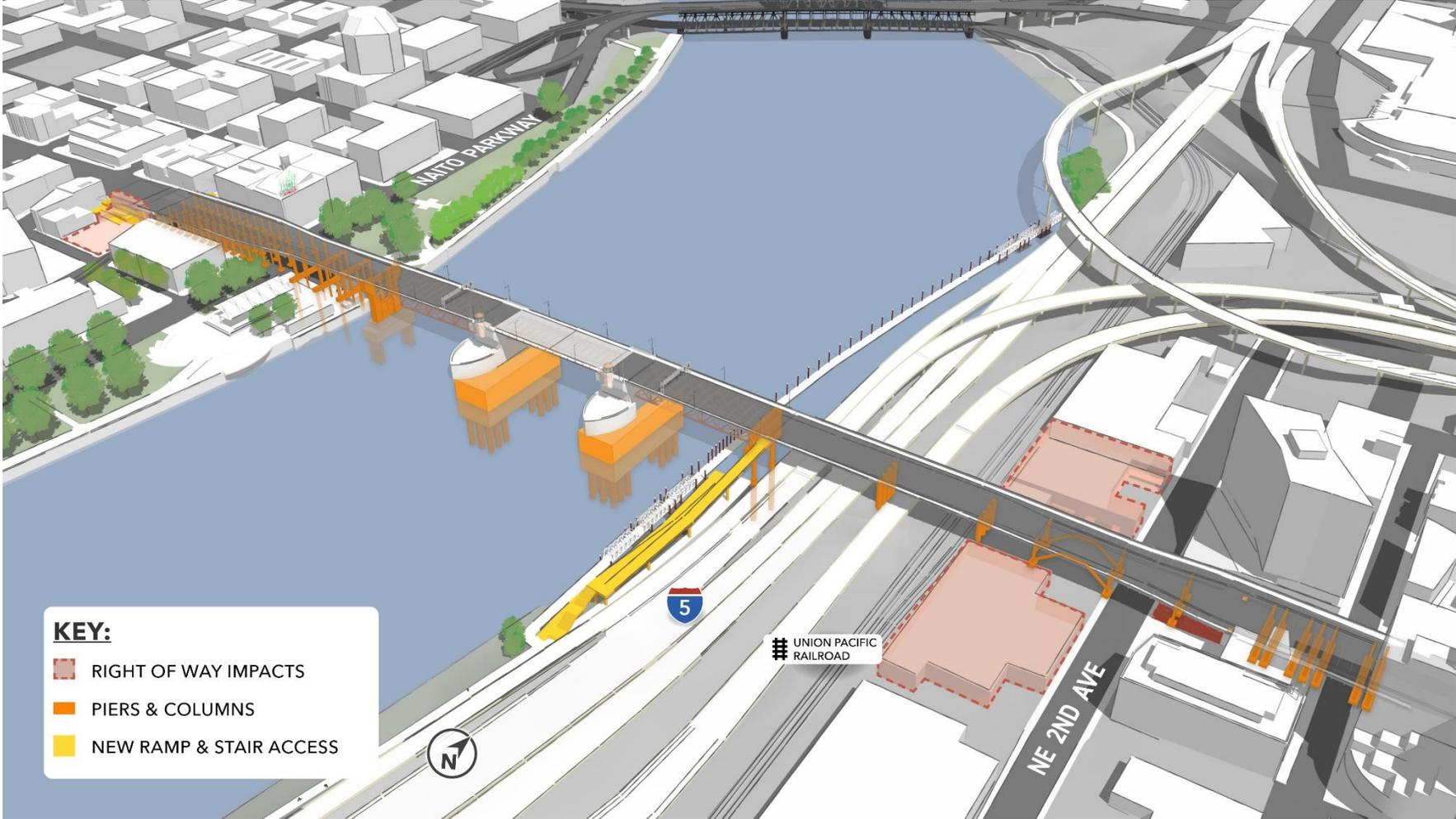
Figure 7. Enhanced Seismic Retrofit – Pier and Bent Locations, Plan View
