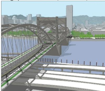
Long-span Alternative / Cable-stayed / Lift
