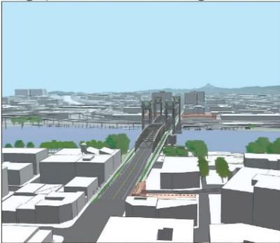
Long-span Alternative / Tied-arch / Lift
