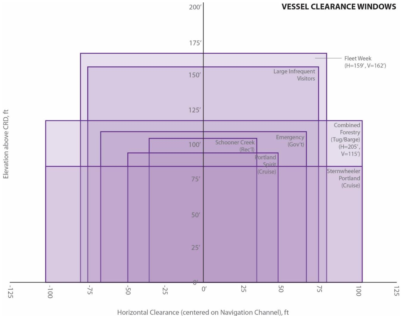
The height and width of each box in Figure 3.2-2 correspond to the required elevation and horizontal clearance (centered on the navigation channel) for each vessel.
